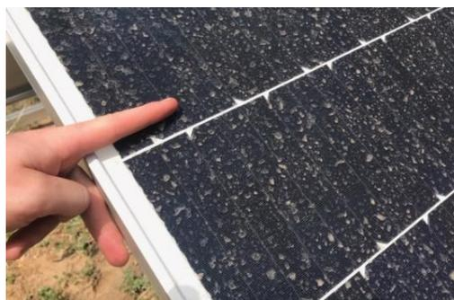
*Figure 1: PV panel with dust soiling*
